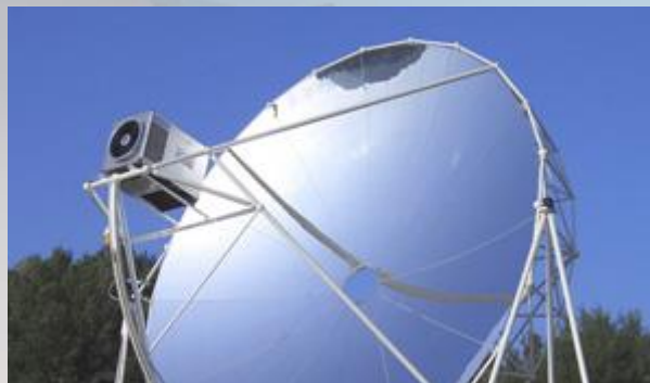
Stirling Engine Generator and Dish
