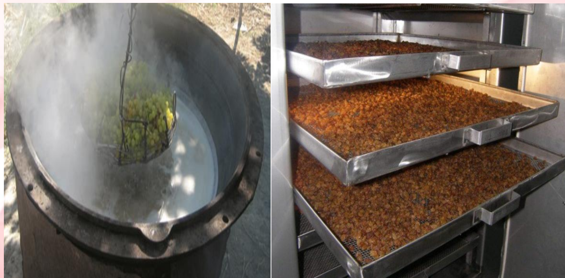
2-rasm. Objo'sh usulida uzumni ishqorli qaynoq suvga botirib, oftobga yoyib quritib mayz olish.
