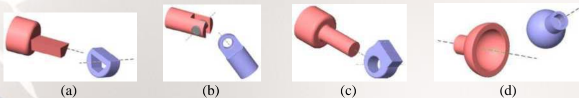
Figure 4. Sketches of disassembled hinges: (a) - Disassembled Prismatic; (b) - Disassembled Revolute; (c) - Disassembled Cylindrical; (d) - Disassembled Spherical.
