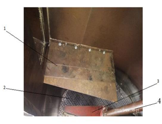
Figure 2. Separator working chamber with a trapezoidal guide. 1- trapezoidal guide; 2 mesh surface; 3-crew, 4-screw shaft.
