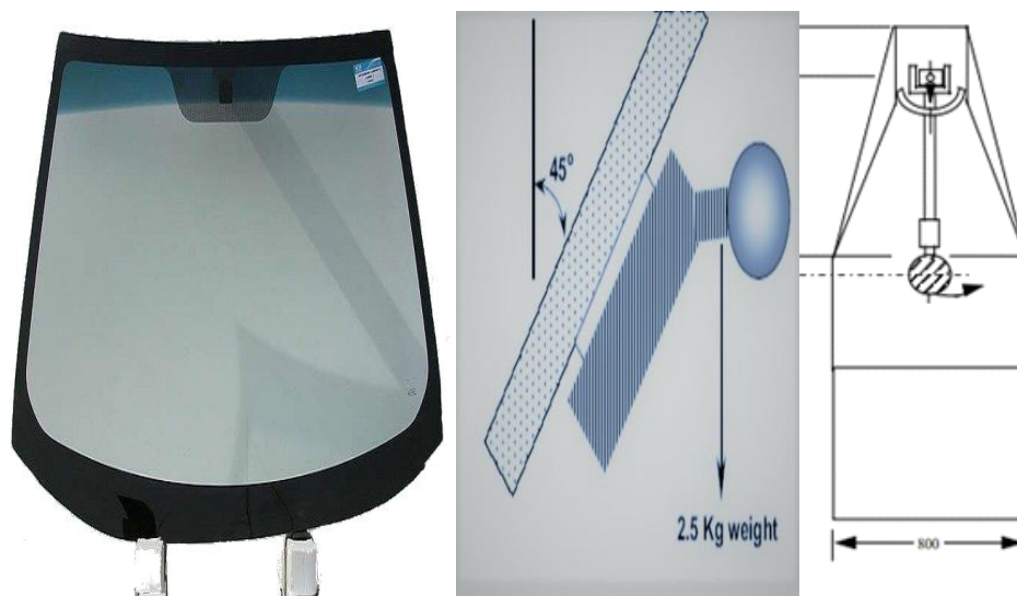
Figure 1 3M structural connecting tape is a scheme for testing the ability to load a plate handle attached to a window.
