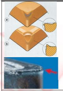
Plastic deformation: a - lowering of the edge; b - deepening of the side surface, leads to poor plate formation and a decrease in machining cleanliness. It increases the risk of serious corrosion of the side, which can lead to failure of the insert.
