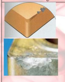
Damage caused by chips falling on the unused part of the cutting edge. The upper and supporting surfaces of the insert may be damaged. When falling, the chips hit the exit side.
